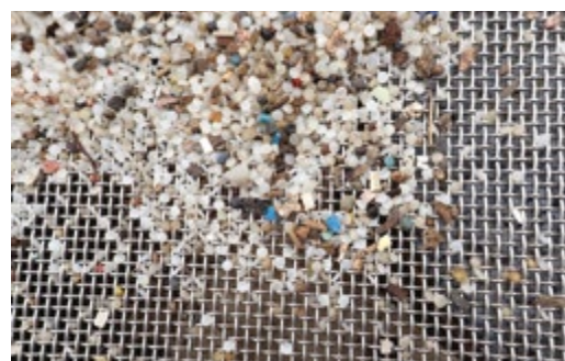
Plastic nurdles spilled from a damaged container are recovered from a beach and sieved to separate the sand to minimise the amount of waste generated – Image courtesy of ITOPF
