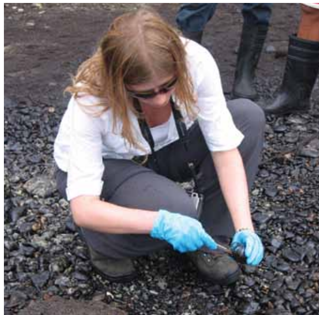
▲ Figure 7: Sampling stranded oil on the shoreline.
