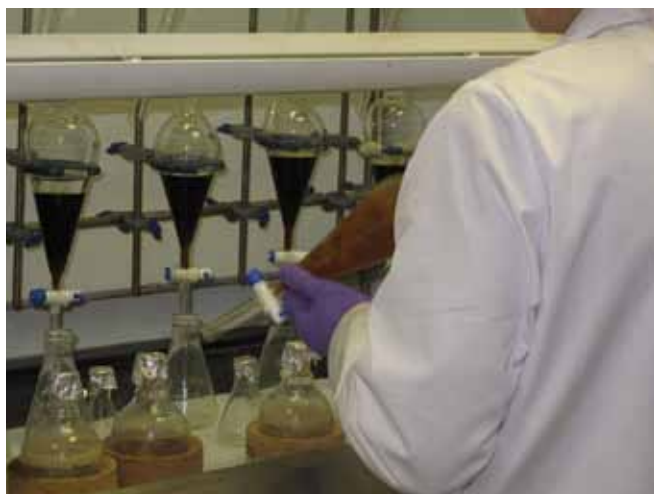
▲ Figure 13: Extraction of oil samples using a separation funnel (image courtesy CEFAS).
