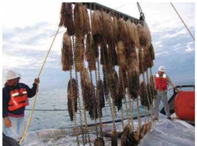
▲ Figure 3: Using sorbents for sub-tidal sampling. The frame, with sorbent attached, is towed along the seabed. The presence of oil on the sorbent when raised allows the geographical extent of sunken oil to be determined.
