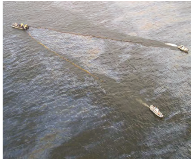
▲ Figure 9: Curtain boom employed in a V configuration by two towing vessels with a separate skimming vessel at the apex.
