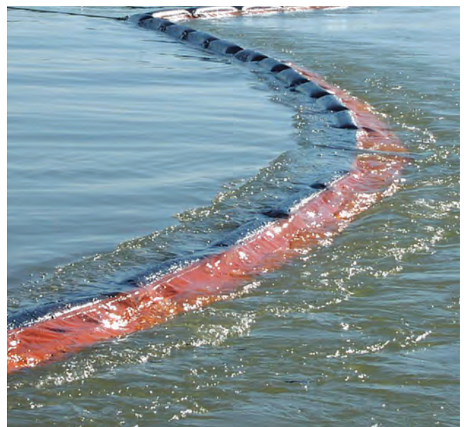
▲ Figure 4: The strong current has caused the boom to plane, allowing any oil to be lost under the skirt.
