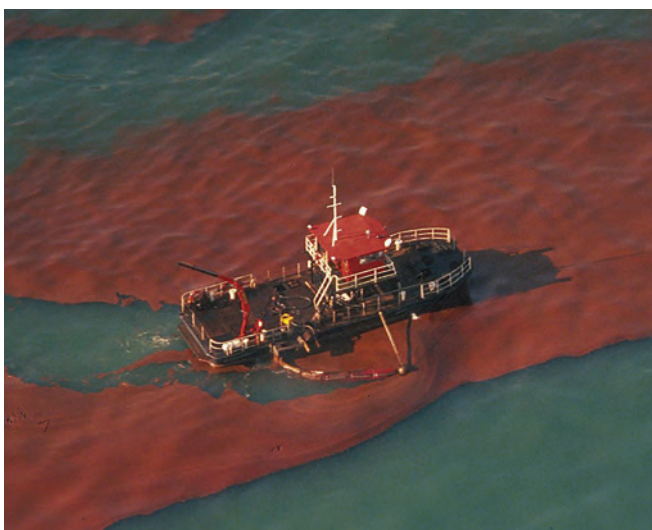
▲ Figure 10: Single ship collection system employing a short length of curtain boom deployed from an oil recovery catamaran, in heavily emulsified crude oil.
