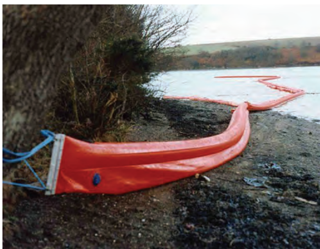
▲ Figure 18: Shoreline sealing boom deployed in an estuary. The lower water ballast chambers allow the boom to sit on the shore at low tide. In this instance, sections of shoreline sealing boom are connected to sections of inflatable curtain boom.
