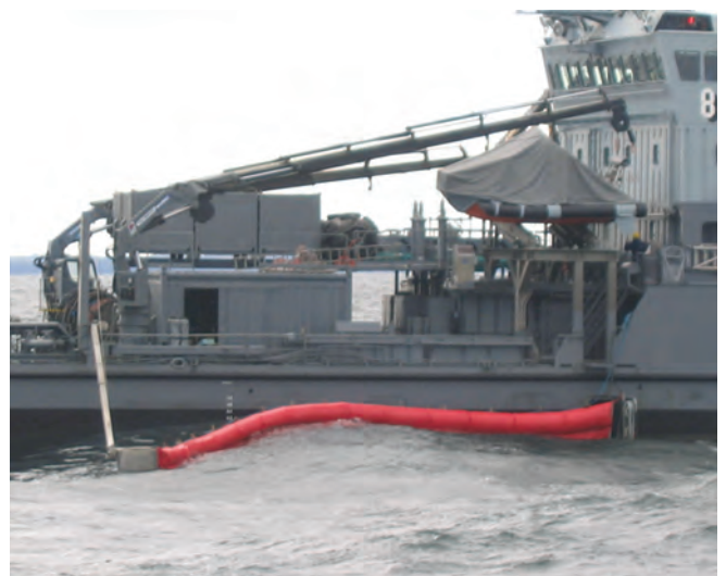
▲ Figure 11: Whilst sufficiently flexible to be able to follow the motion of the waves, the boom has risen from the water where it attaches to the hull, potentially allowing oil to escape from the apex.
