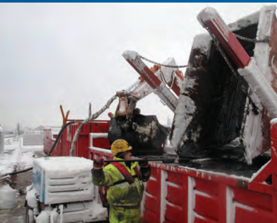
Cold conditions made it necessary to heat recovered oil prior to transportation, Liverpool Docks, UK
